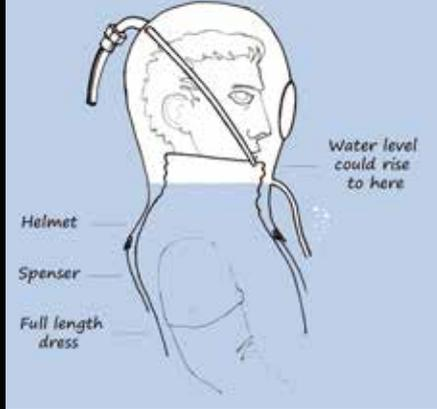
Siebe's tube brought air in front of the diver's mouth. This meant that an interruption in the airflow could allow water to rise as high as the helmet volume.
