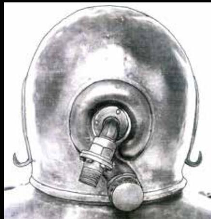
Edward's circuitous exhaust valve, with the air inlet at its centre.
